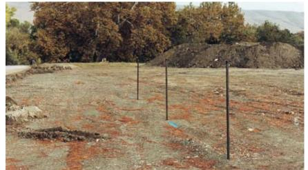
Listen directly over the pipe between these two loudest locations. Use your hearing and the meter to determine exactly where the leak sound is loudest:
