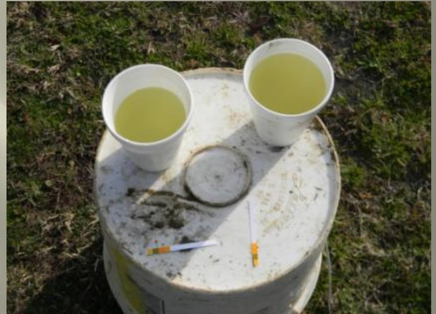
After nearly 30 minutes of pumping, the color started staying a consistent green. We charted the change in color from time to time. By the time it reached this color, the pH level was never less than 7.0
