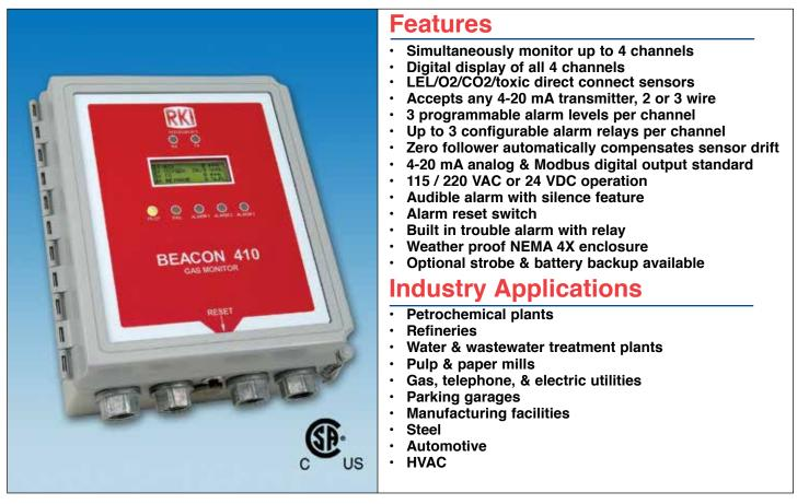
The Beacon 410 is a highly configurable, microprocessor-based, flexible and easy to use 4 channel gas monitor. It simultaneously displays the gas type, readings, and status for 4 channels of gas detection. It can monitor any combination of direct connect sensors (LEL combustibles, oxygen, CO2, and toxic gas sensors, as well as any 4-20mA transmitters.
