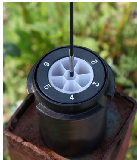
Measure Water Levels within the narrow channels of a Solinst CMT® System.
