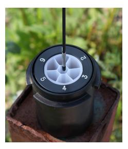
Measure Water Levels within the narrow channels of a Solinst CMT<sup>®</sup> System.
